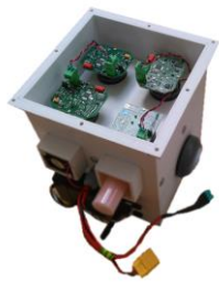
BH-8, Ultra light gas sensor package
